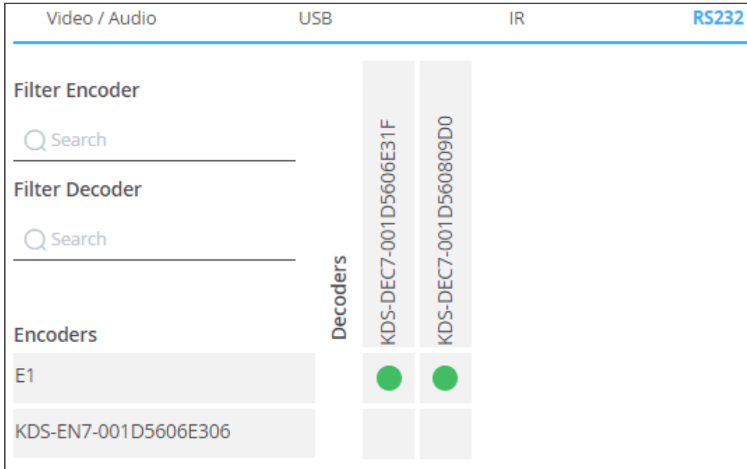
Figure 21: Routing an RS-232 Signal
